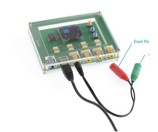
Pressing the orange mode button (**A** in first image) can toggle Edit and Menu modes. To edit the selected item in navigation mode, toggle the mode into edit mode, then use the UP and DOWN (B and C button in first image) to change the value of it.
