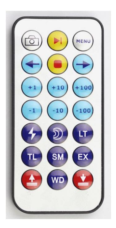
There are 21 buttons on the remote control. When screen is turned off, any press of button on the remote control will turn the screen on without doing anything else.
