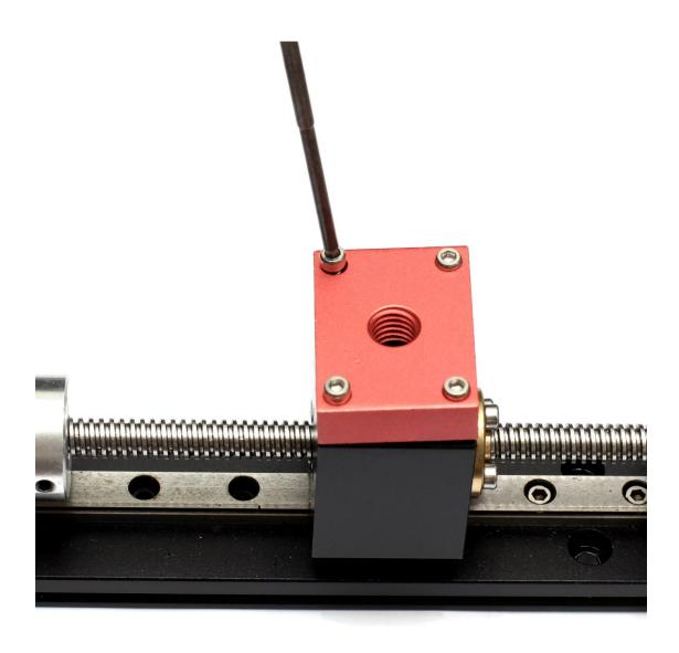
**Step Two**: Put camera quick release on to the rail so that any camera with quick release plate can be slided in and secured.
