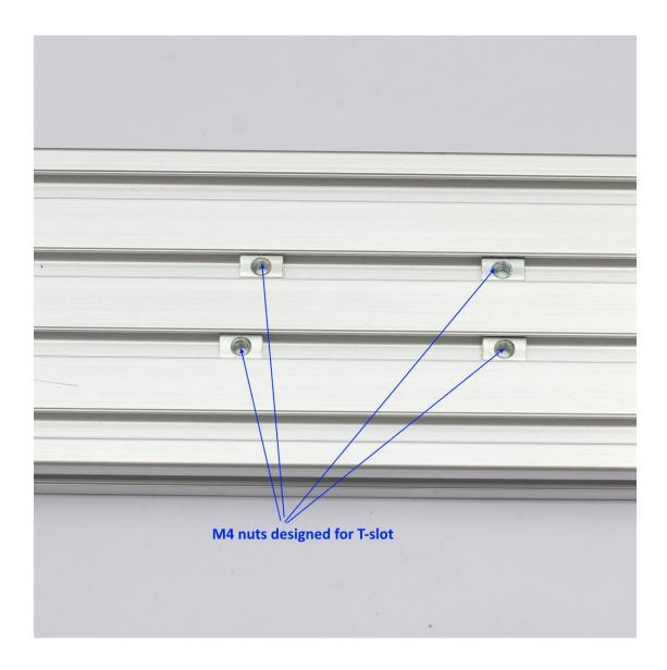
Put the rail on top of the T-slot and align it so that mounting holes on the rail is right on top of each nuts, then use M4 screws to secure the rail. There are six mounting holes, you can use the front 4, the other two is kind hard to access.
