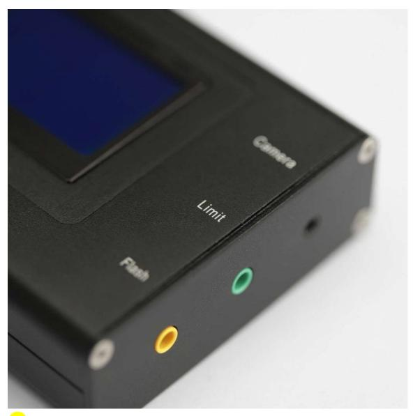
Flash Port – this is where a flash or continuous light can be plugged in. Parameters for this port can be set in Time menu by pressing
