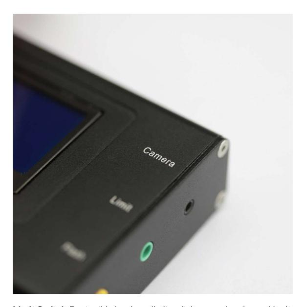
**Limit Switch Port** – this is where limit switches can be plugged in. It is a 3.5mm stereo socket and supports two limit switch inputs. The two limit switches can be installed at each end of the rail. The base ring of 3.5mm plug is the common ground shared by the two limit switches. The middle ring and the tip are the two limit switches.
