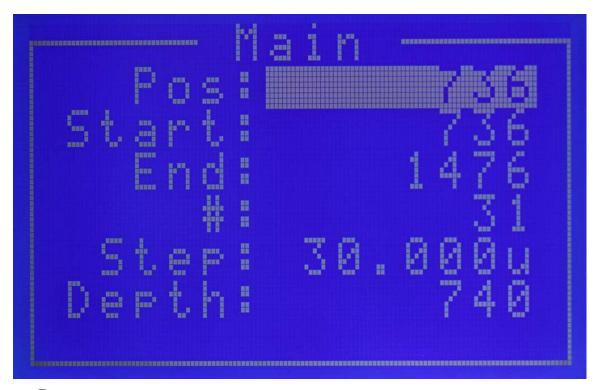
Pos – this is the current position of the rail. When it is high lighted, pressing -100 or +100 button will move the rail by 100,000 steps backwards or forwards respectively, essentially moving the rail until STOP button is pressed. Pressing -1 or +1 button will move the rail by one step size backwards or forwards. Pressing -10 or +10 button will move the rail by 10 step sizes either backwards or forwards.
